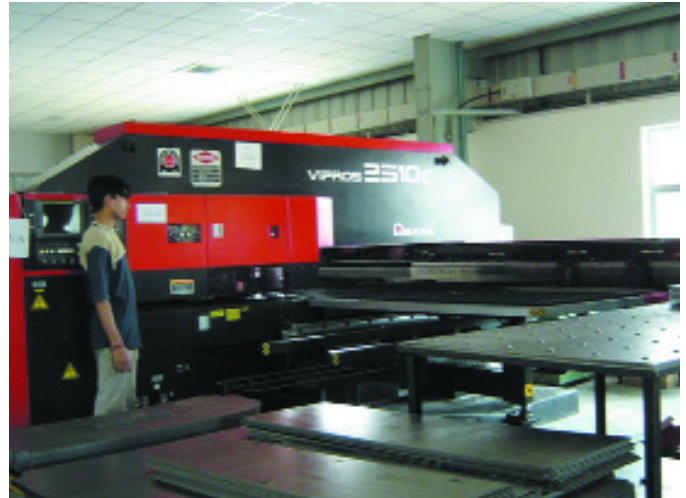
CNC turret punch and press brakes for accuracy in punching, bending and shearing
