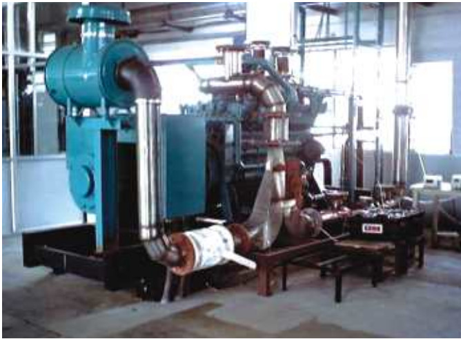
GTA-1710-G Cummins engine operating on 100% producer gas
