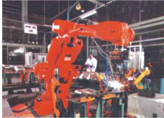
Robotic welding at the H-One India Weld Shop
